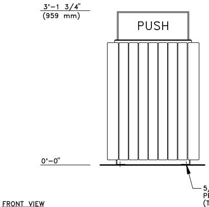
5/8" (16 mm) DIAMETER HOLES PROVIDED FOR ANCHORS BY OTHERS. (TYPICAL-4)
